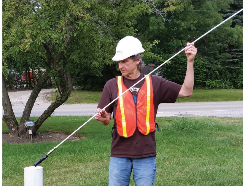
Fit rod into well casing. Stop when piston reaches bottom.
