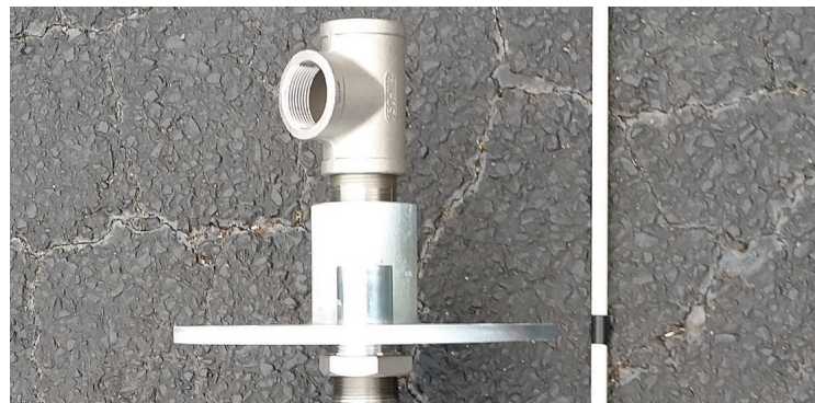
Discharge tee, well seal, pipe nipple, drive rod.
