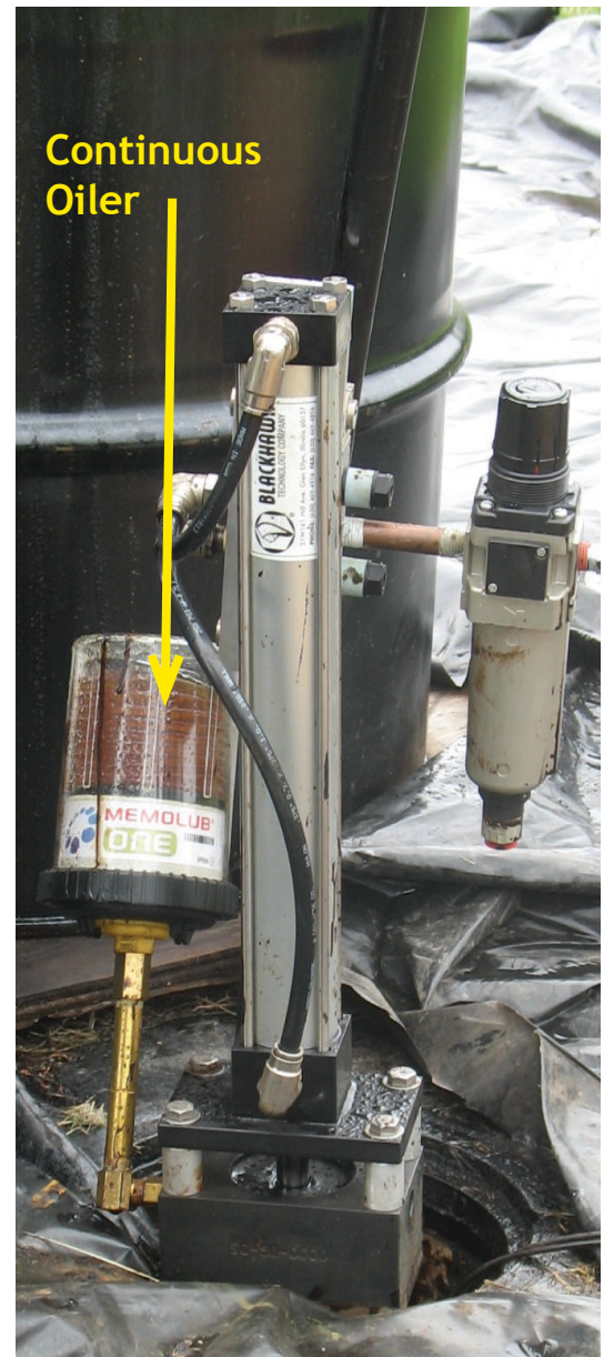
Continuous rod oiler attaches to seal plate
