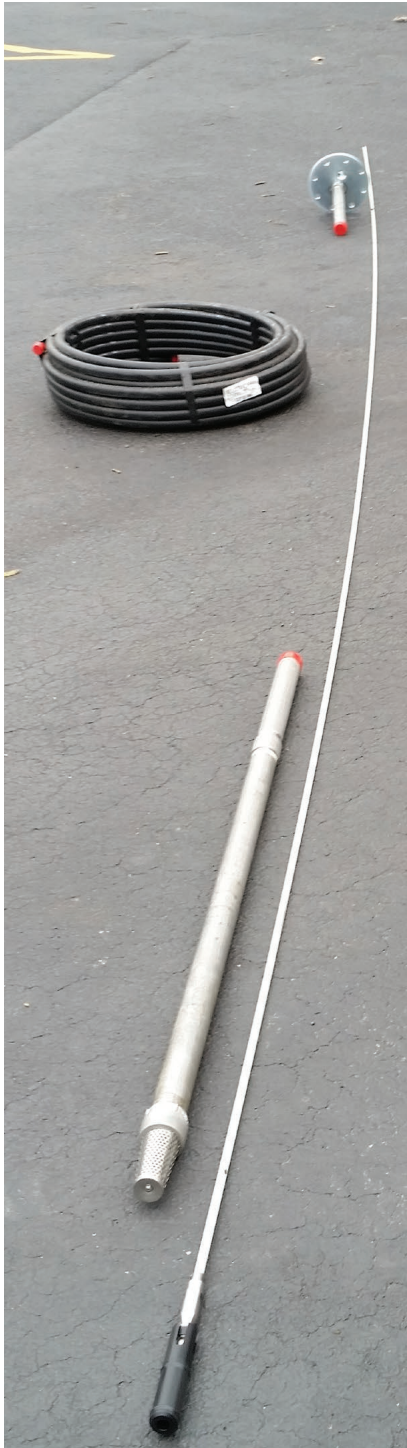
Lay out piston, drive rod, well seal and discharge tee. At left are foot-valve assembly and coiled HDPE riser pipe.
