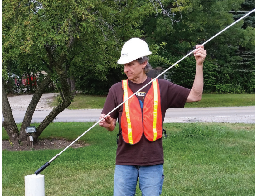
Fit rod into well casing. Stop when piston reaches bottom.
