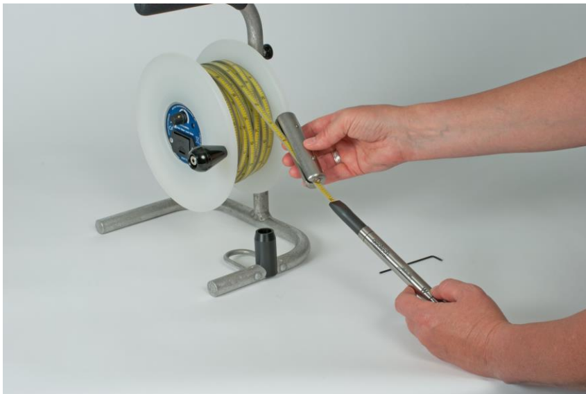
Figure 2-2: Fitting (Optional) Tape Weight
