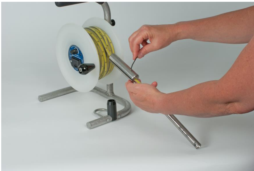
Figure 2-3: Tightening (Optional) Tape Weight
