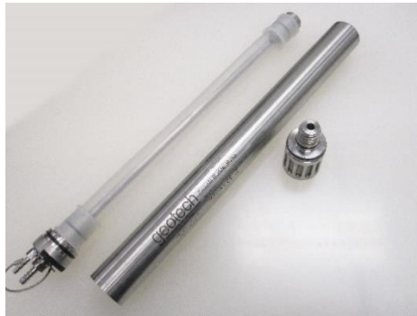
Figure 4-1: Removal of the bottom intake and outer housing
