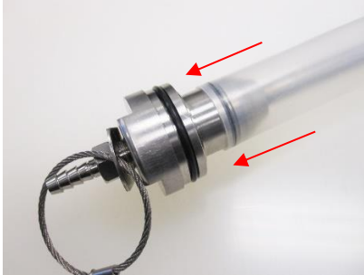
Figure 4-13a: Sliding bladder on
