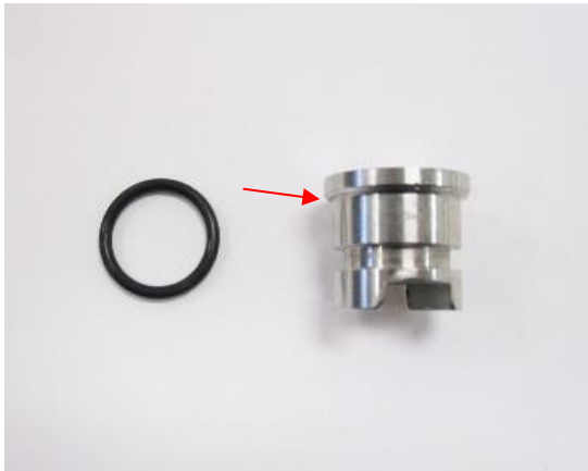
Figure 4-8: Check Ball Retainer O-ring
