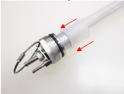
Figure 4-14a: Compression Ring on Bladder
