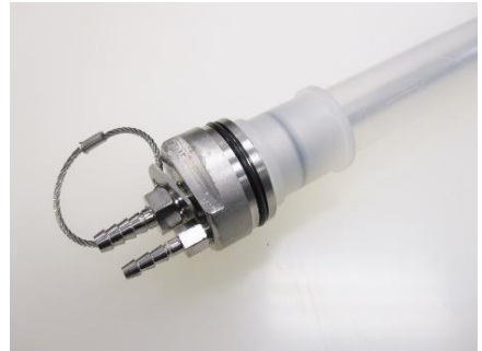
Figure 4-14b: Compression ring secured
