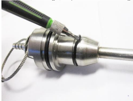
Figure 4-5: Removal of O-rings
