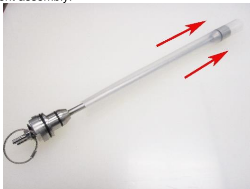
Figure 4-4: Removal of Bladder
