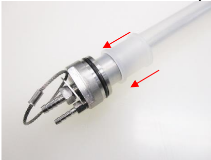
Figure 4-14a: Compression Ring on Bladder
