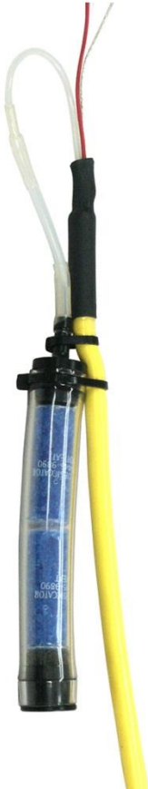
Figure 1-2: Example of Desiccant Pack installed on Vented Transducer cable.
