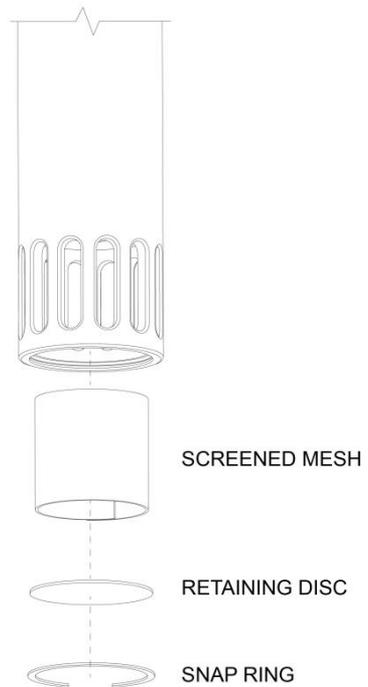
**Figure 4-1:** Screened Intake Components
