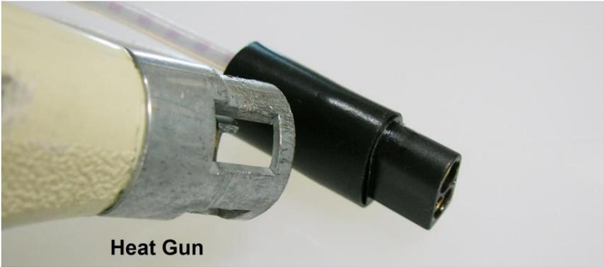
**Figure 4-5: Heating the Heat Shrink**
