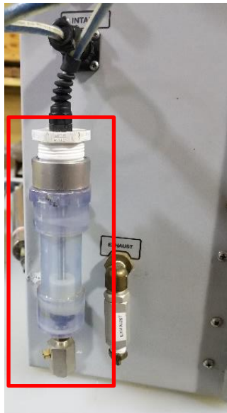
Figure 5-10: Intake Float Switch
