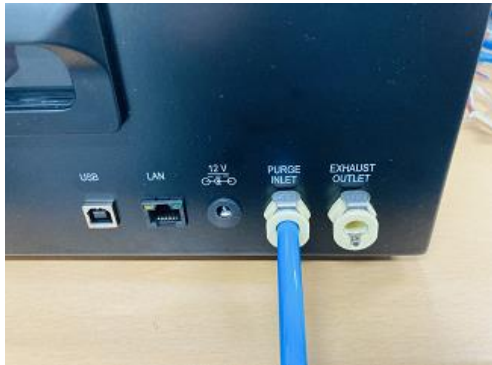
Purge Inlet - 1/8" Tube connect to Clean Air
