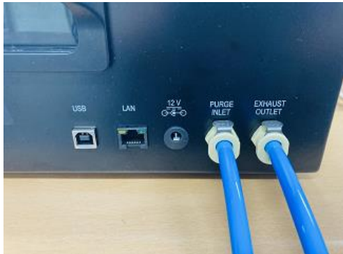
Exhaust Outlet - 1/8" Tube connect to Ventilation
