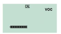
Press and hold the multi-function button until the Cub beeps then release it quickly to avoid switching it off.
