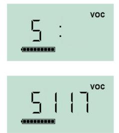
Press the multi-function button to initiate the Span stage. The screen will display an 'S'.
