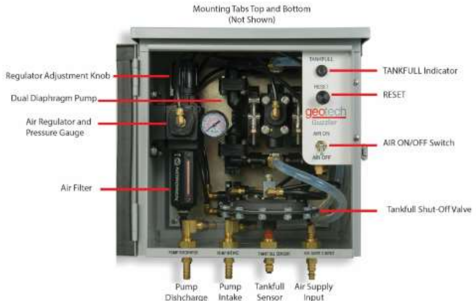
Figure 2-1: Guzzler Control Box Components
