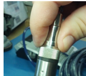
Properly completed—black ring uncompressed
