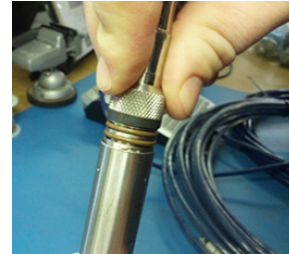
Push top cap in before twisting and locking
