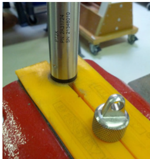
Cableless Sensor—gripping on knurled area
