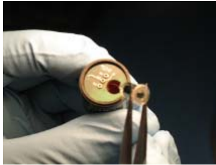
Figure 7–10. Installing the Lamp into the Sensor
