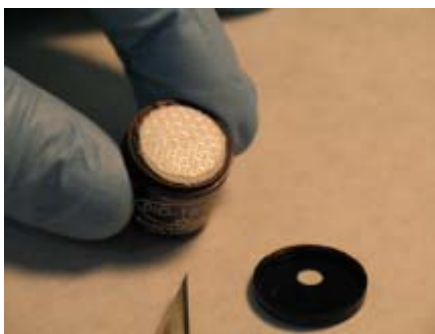
Figure 7-5. Removing the Filter Media
