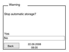
2 Using <▲><▼>, select Yes and confirm with <ENTER>. The measuring instrument switches to the measured value display.
