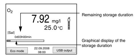
The active automatic storage function can be recognized by the progress bar in the status line. The progress bar indicates the remaining storage duration.
