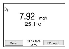
2 Using **<F1**\_\_>/[Menu] open the *Storage & config* menu. The instrument is in the setting mode.
