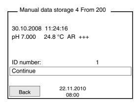
2 If necessary, change and confirm the ID number (1 ... 10000) with <**△**><**▼**> and **<ENTER**>. The dataset is stored. The meter switches to the measured value display.
