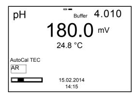
21. Wait for the measurement with stability control to be completed or terminate the stability control and take over the calibration value with <ENTER>.
