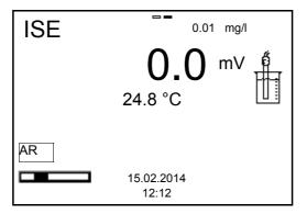
11. Wait for the end of the AutoRead measurement or accept the calibration value with **<ENTER>**.
