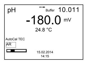
9. Wait for the end of the measurement with stability control or accept the calibration value with **<ENTER>**.
