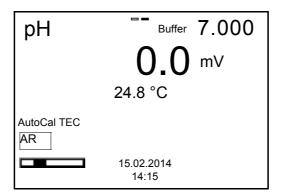
15. Wait for the measurement with stability control to be completed or terminate the stability control and take over the calibration value with <ENTER>.
