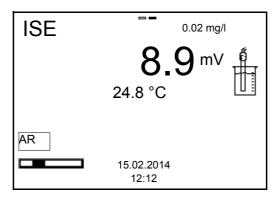
16. Wait for the end of the AutoRead measurement or accept the calibration value with **<ENTER>**.
