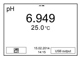
2. Using **<ENTER\_\_>**, open the *Storage & config* menu. The instrument is in the setting mode.
