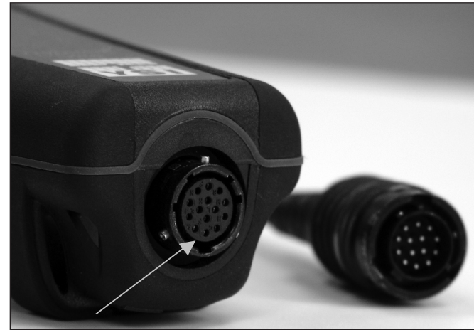
Figure 4, Note the keyed connector.
