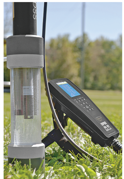
ProDSS attached to Tripod and Flow Cell for groundwater applications
