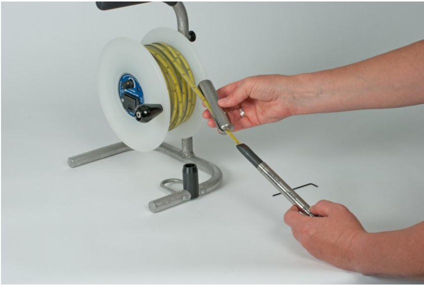
Figure 2-2 Fitting (Optional) Tape Weight
