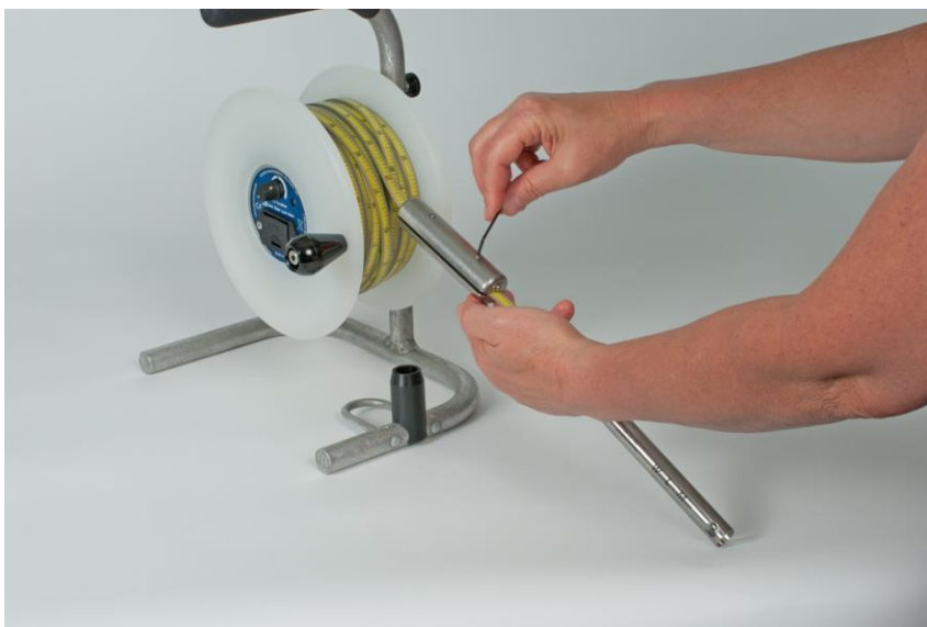
Figure 2-3: Tightening (Optional) Tape Weight
