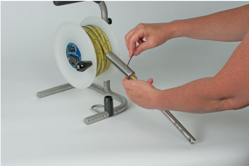
Figure 2-3 Tightening (Optional) Tape Weight
