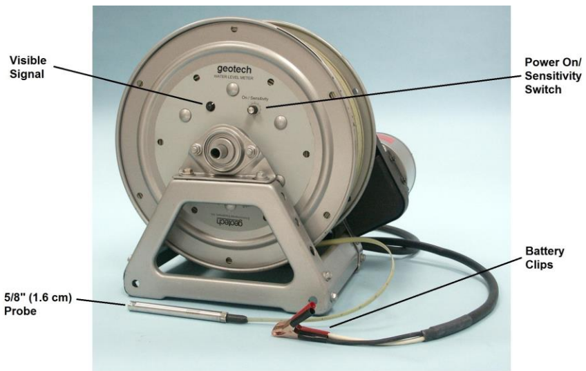
Figure 1-3: Electric Reel Front View
