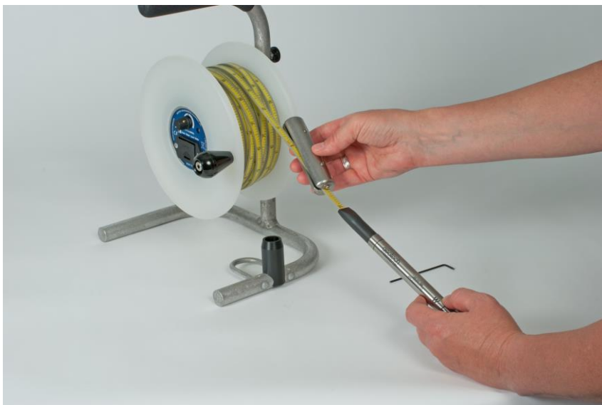
Figure 2-2: Fitting (Optional) Tape Weight
