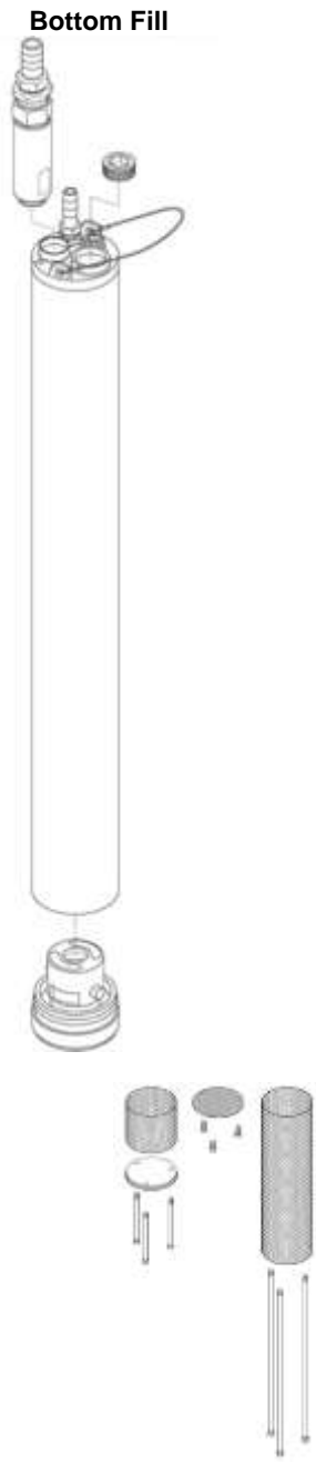
Figure 4-1: Top and Bottom Fill Reclaimer
