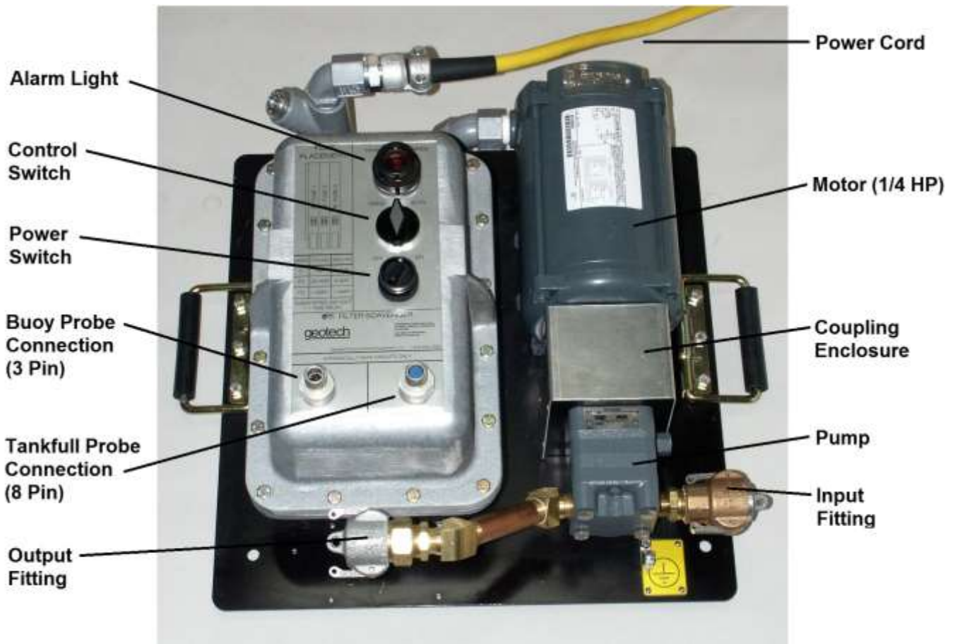
Figure 1-3: LDFS Pump Control Module Assembly
