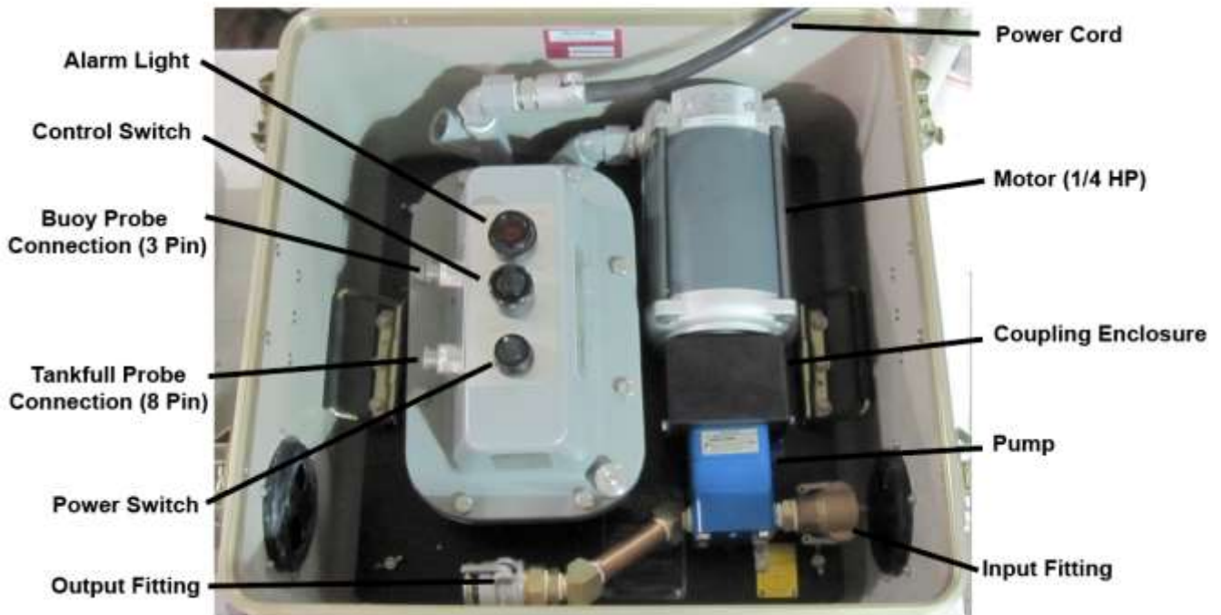
Figure 1-4: New LDFS Pump Control Module Assembly
