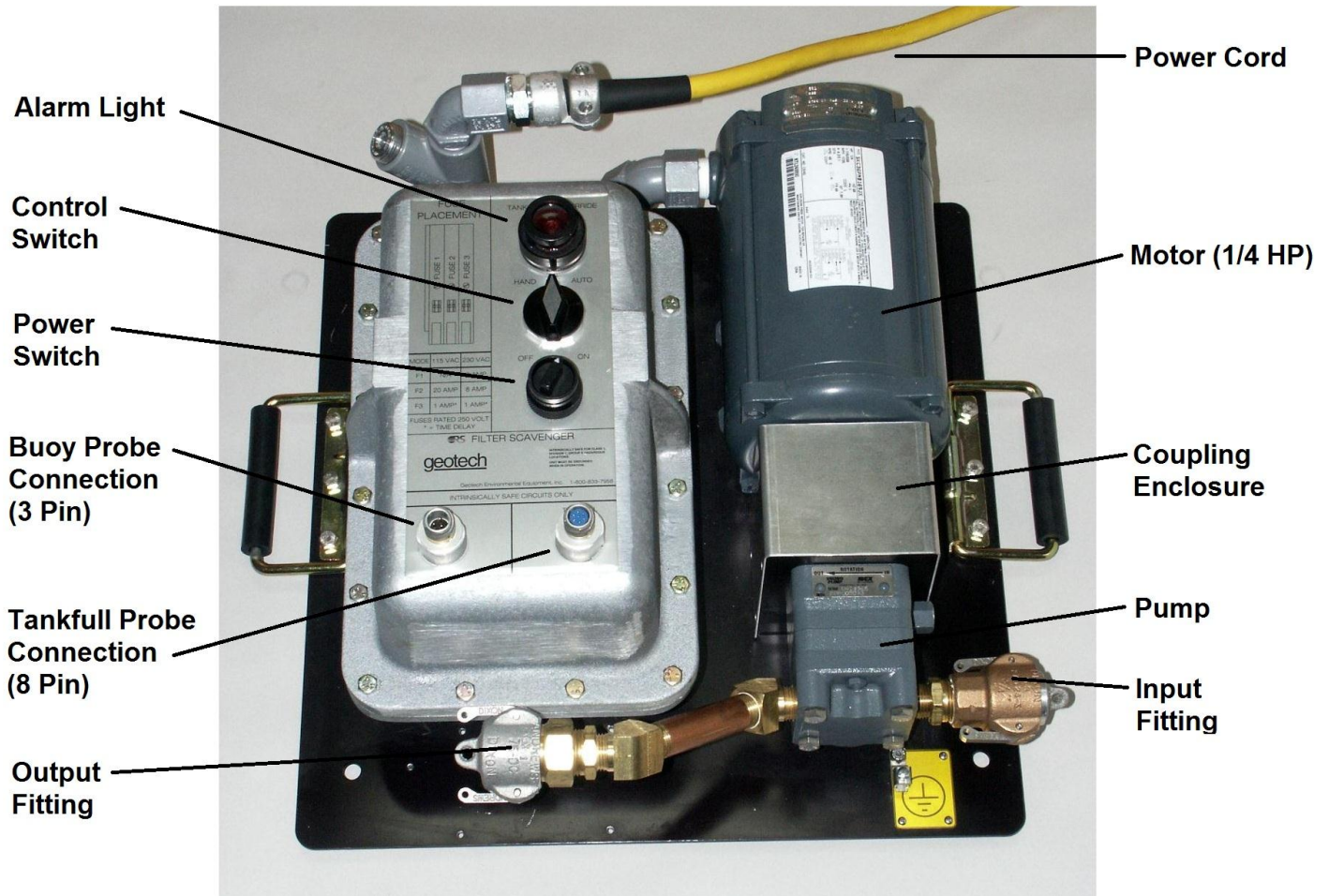
Figure 1-3 - LDFS Pump Control Module Assembly
