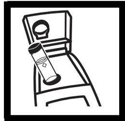
**6.** Insert the **second** sample cell into the cell compartment and close the cover.
