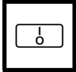
**3.** Press: I/O to turn the instrument on.
