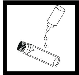
**1.** Collect a representative sample in a clean container. Fill a sample cell to the line (about 15 mL), taking care to handle the sample cell by the top. Cap the cell. (See *Section 2.3* on page 22 for more information about collecting a representative sample).
