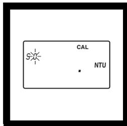
**1.** Rinse a clean sample cell with dilution water several times. Then fill the cell to the line (about 15 mL) with dilution water or use StablCal <0.1 NTU standard.
