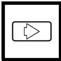
**15.** Edit the standard concentration by pressing **→**. The **3** will stop flashing and the left digit in the display will flash. Press **↑** to scroll the digit up to the appropriate number. Press **→** again to move the cursor to the next digit and edit it in the same manner.
