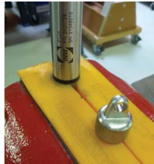
Cableless Sensor - gripping on knurled area
