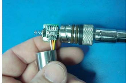
Connector connected properly
