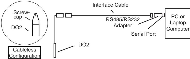
*Connect the DO2 to your computer using an RS485/RS232 adapter and an interface cable.*
