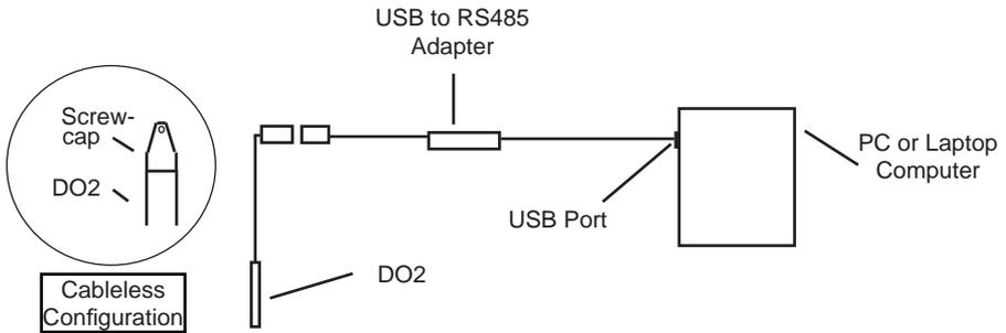
*Connect the DO2 to your PC using a USB to RS485 adapter.
