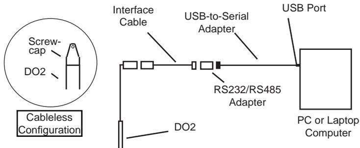
*Connect the DO2 to your computer using a USB to Serial adapter and an interface cable.*
