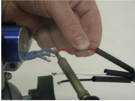
After all connections are soldered, apply heat shrink to cover all connections.
