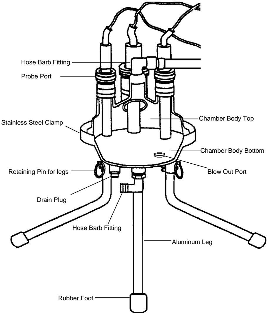
The probe chamber accepts up to five probes simultaneously. Four of the ports accommodate probes from  $\frac{1}{8}$ " to  $\frac{5}{8}$ " in diameter. The fifth port can accommodate from  $\frac{3}{4}$ " to 1". Any or all ports can be plugged off with a PTFE blank when not in use. Each port contains:
