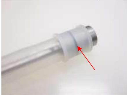
**Figure 4-15:** Bottom Compression ring with visible O-ring
