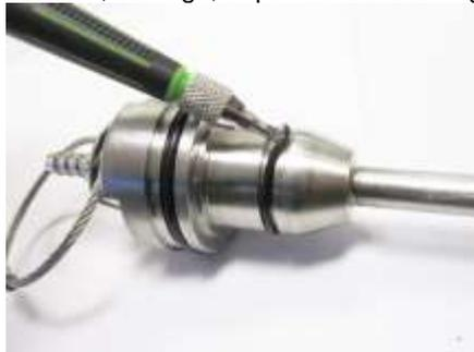
**Figure 4-5:** Removal of O-rings
