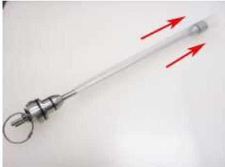
**Figure 4-4:** Removal of Bladder
