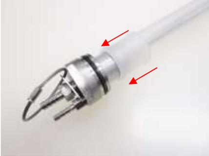
**Figure 4-14a:** Compression Ring on Bladder
