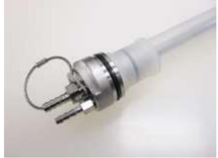
**Figure 4-14b:** Compression ring secured
