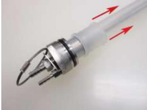
**Figure 4-3:** Removal of upper HDPE Compression Ring
