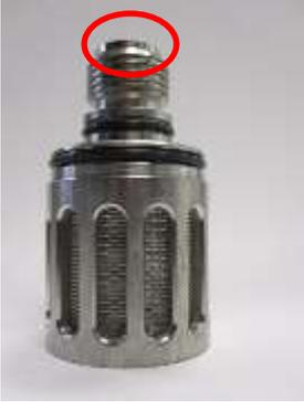
**Figure 4-7a:** Check Ball Retainer
