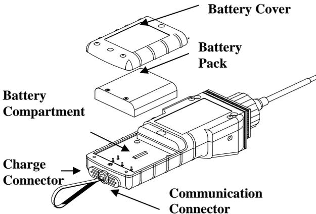
**Figure 6-1 Battery Replacement**
