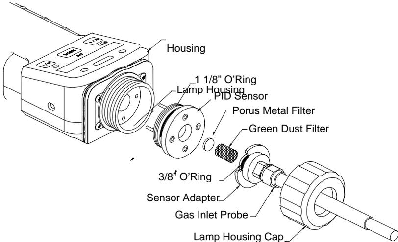
**Figure 7-2 Sensor Components**
