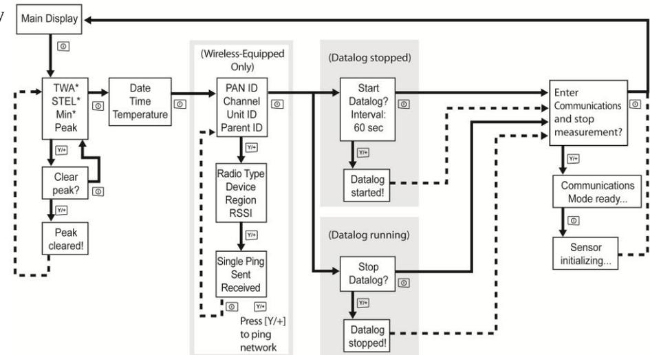
\* If your ToxiRAE Pro is configured with an oxygen (O<sub>2</sub>) sensor, TWA and STEL are not included in the menus because neither TWA nor STEL are calculated for this sensor. Min (for minimum) is included only when an oxygen sensor is used.
