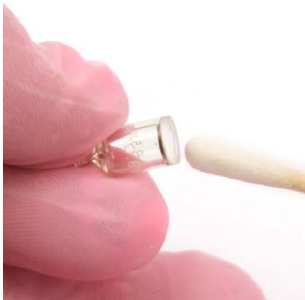
Figure 31: Polishing the Electrode Lamp Window
