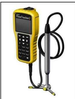
The FlowTracker2 measures velocities with a range as low as 0.001 m/s (0.003 ft/s) and up to 4.0 m/s (13 ft/s). When combined with a wading rod, the FlowTracker2 can be used to measure the total discharge across a river section.
