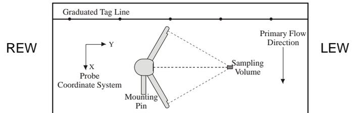
Based on the depth, station width, and mean velocity, the discharge for a station is calculated. The total discharge is the sum of all station and edge discharge values.
