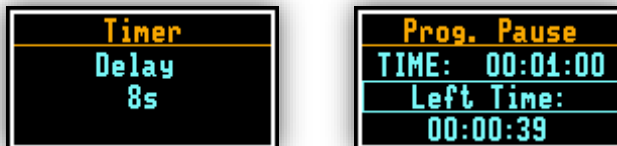
Figure 4-18 Auto-run mode – timer and programmable pause screen
