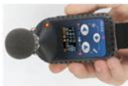
Figure 2-1 SV 104A instrument with the microphone and windshield
