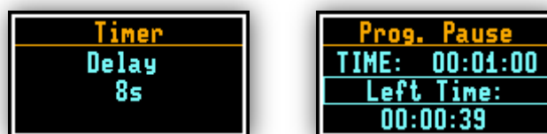
Figure 4-18 Auto-run mode – timer and programmable pause screen
