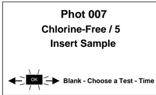
Place **SAMPLE TUBE** (sample and reagent) in the test chamber, then press **[OK]**.
