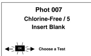
Place a **BLANK TUBE** in the test chamber, then press [OK].
