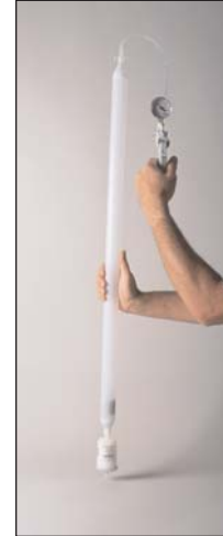
In-line filtration using the Geotech Hand Pump, pressurized bailer and dispos-a-filter™
