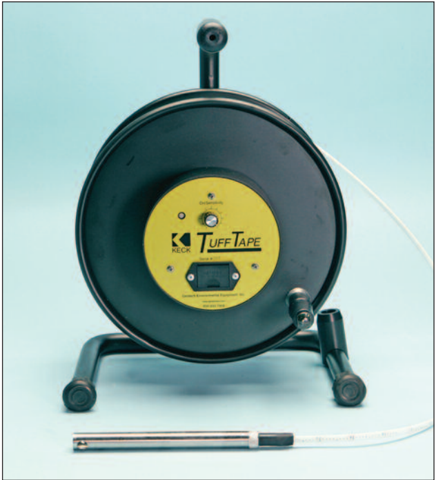
Keck Tuff Tape™ Water Level Meter
