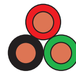
2-wire with ground, twisted
