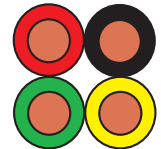
3-wire with ground, twisted
