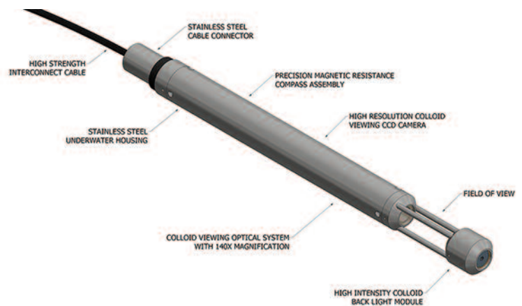
Borescope Probe Detail
