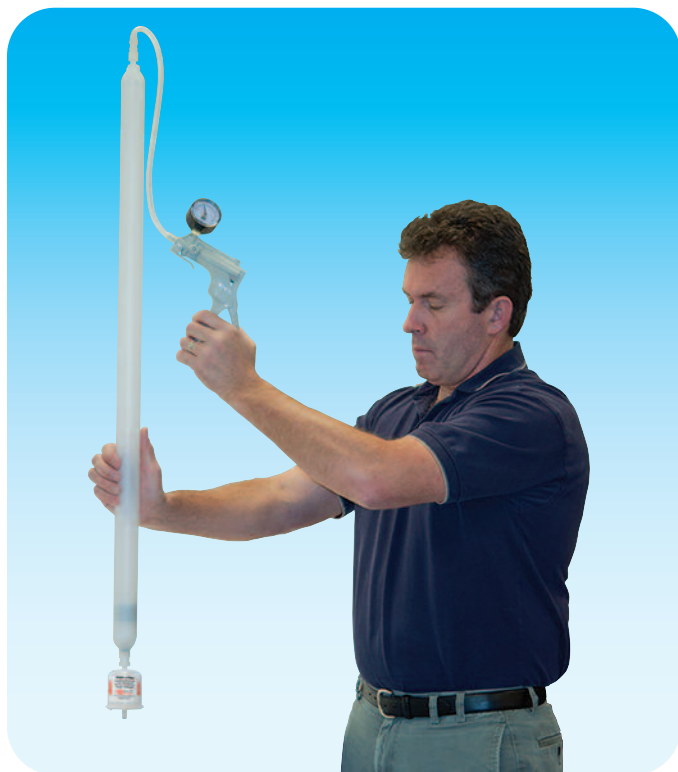
In-line filtration using the Geotech Hand Pump, pressurized bailer and dispos-a-filter™
