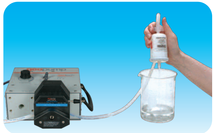
Sample collection with the Geopump™ Peristaltic Pump and dispos-a-filter™ capsule sold separately
