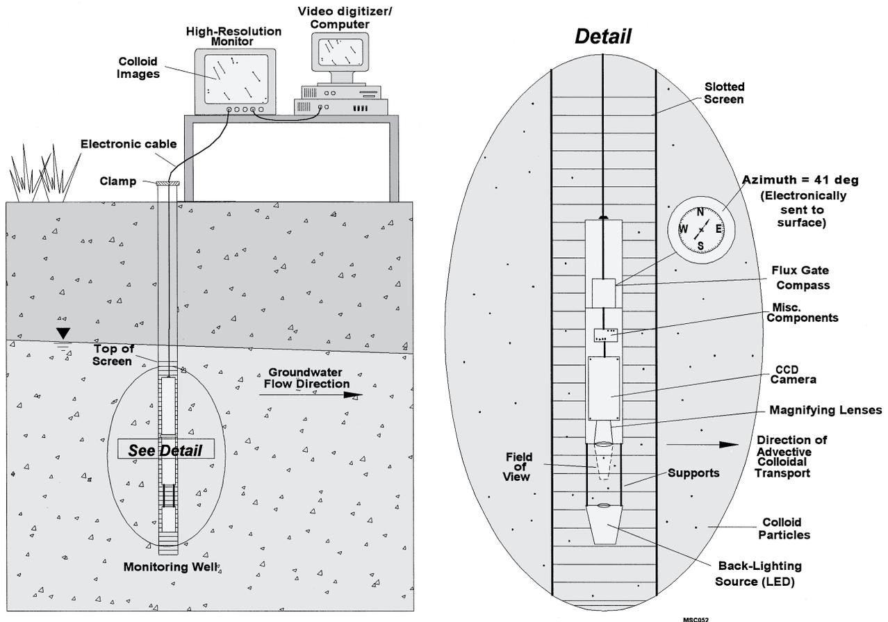
Figure 1. Conceptual diagram of the colloidal borescope.
