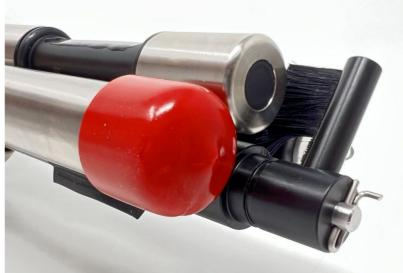
using RapidCal or using buffers containing interfering ions (i.e. all other ISE calibration solutions other than the one for the specific ISE being calibrated and EC calibration solutions) in order to protect the ISE electrodes from the effects of the buffer solution or interfering ions. At all other times, the ISE electrodes should be left uncovered.
