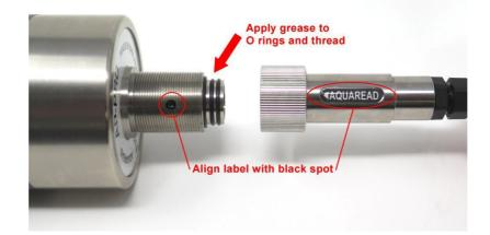
Apply a generous smear of grease to the O-rings where indicated above. Be careful not to get any grease inside the connector near the gold contacts. A small smear of grease should also be applied to the thread on the Probe to allow easy tightening of the collar.
