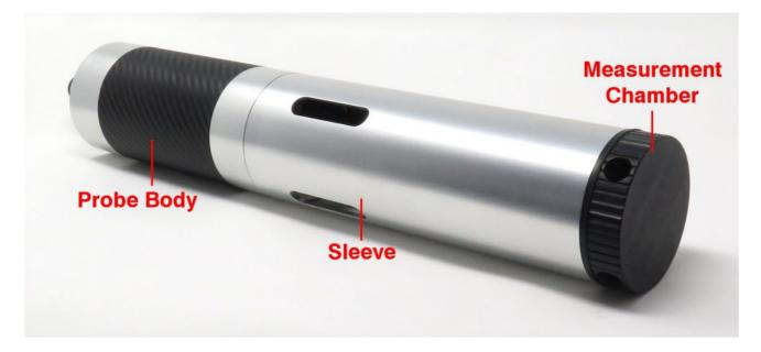
The Sleeve, complete with Measurement Chamber can be easily removed from the Probe Body by unscrewing to allow cleaning of the individual electrodes. Likewise, the Measurement Chamber can be removed from the Sleeve to allow cleaning. See image below.
