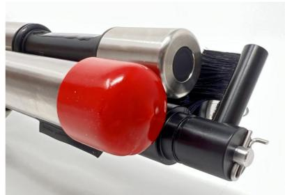
The caps should be fitted to all ISE Electrodes during pH/ORP calibration, when using RapidCal or using buffers containing interfering ions (i.e. all other ISE calibration solutions other than the one for the specific ISE being calibrated and EC calibration solutions) in order to protect the ISE electrodes from the effects of the buffer solution or interfering ions. At all other times, the ISE electrodes should be left uncovered.
