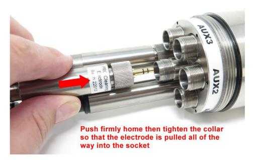
To fit the new cleaning electrode, simply reverse this procedure ensuring the gold contacts on the plug are clean. No special alignment is necessary.
