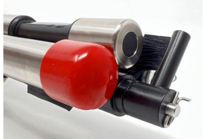
The caps should be fitted to all ISE Electrodes during pH/ORP calibration, when using RapidCal or using buffers containing interfering ions (i.e. all other ISE calibration solutions other than the one for the specific ISE being calibrated) in order to protect the ISE electrodes from the effects of the buffer solution or interfering ions. At all other times, the ISE electrodes should be left uncovered.
