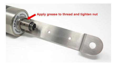
During deployment, the AP-Pro<sup>™</sup> **should not** be suspended by the Extension Cable. A non-conductive Mylar or Nylon cord should be attached to the mounting bracket and be used to support the weight of the AP-Pro<sup>™</sup>.
