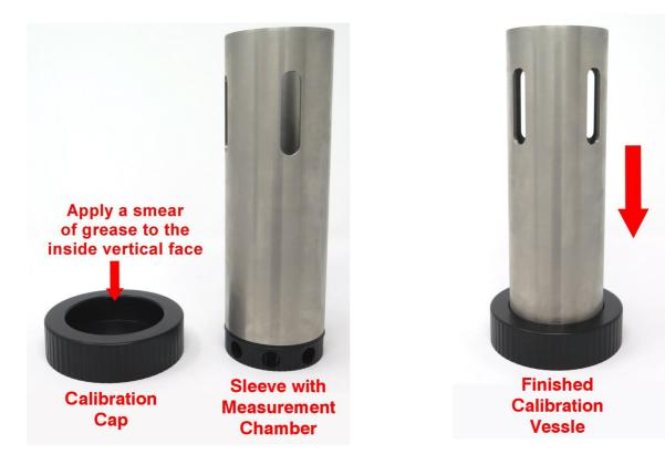
The calibration vessel is now ready for use and should be used for all calibration operations.
