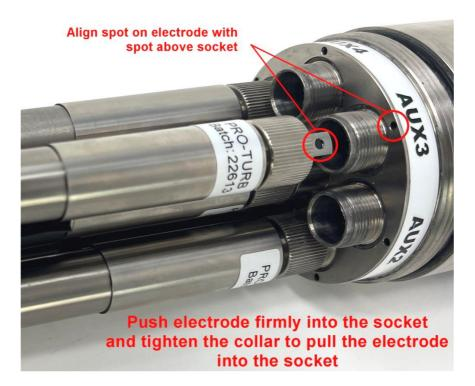
Tighten the knurled collar until the electrode is pulled all the way into the socket.
