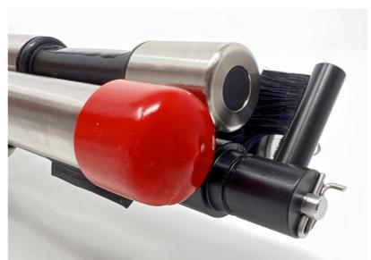
The caps should be fitted to all ISE Electrodes during pH/ORP calibration, when using RapidCal or using buffers containing interfering ions (i.e. all other ISE calibration solutions other than the one for the specific ISE being calibrated and EC calibration solutions) in order to protect the ISE electrodes from the effects of the buffer solution or interfering ions. At all other times, the ISE electrodes should be left uncovered.
