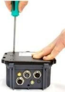
9. Tighten the six back panel screws with a torque of 1 Nm. Do not over-tighten because it will strip the screw threads.
