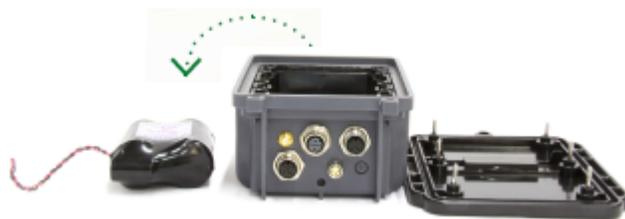
5. Carefully disconnect the male end of the battery connector cable from the female connector on the interface board. Using an indelible pen, mark the battery as "Used" and dispose of it properly.
