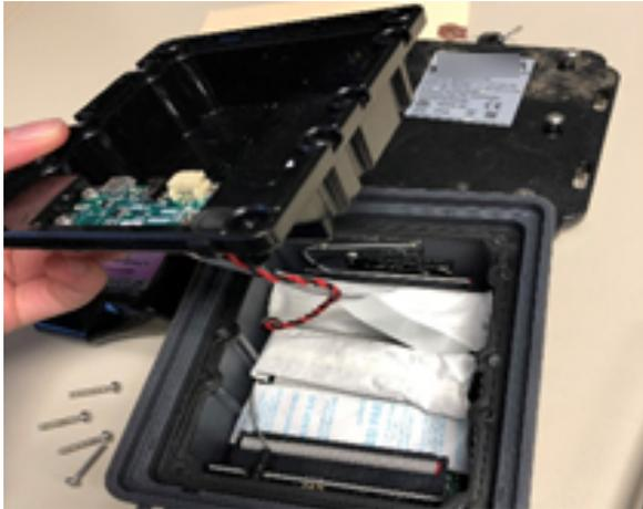
5. Unplug the red and black wires from the underside of the plastic casing to allow easier access to the SIM card. Set the casing to the side.
