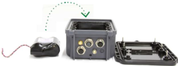
6. Mark the new battery with the current date. Place the battery in the device enclosure and carefully connect the male end of the battery connector cable to the female connector on the interface board.
