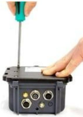
2. Partially unscrew the six (6) screws located on the back of the device enclosure, until you can lift off the back panel with the screws still affixed to their screw holes.
