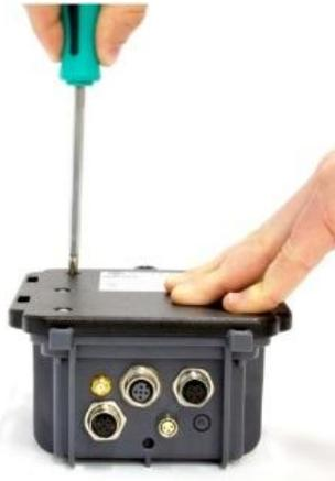
8. Tighten the six back panel screws with a torque of 1 Nm. Do not over-tighten because this will strip the screw threads.
