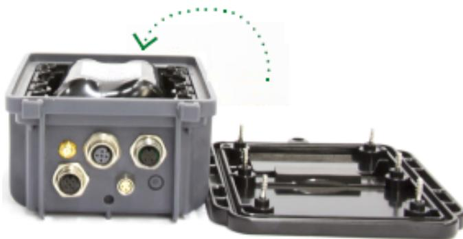
7. Replace the device's back panel, ensuring that the battery cable is neatly arranged and not pinched within the device enclosure.
