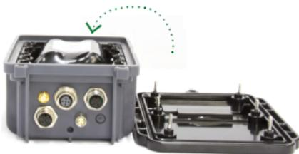
8. Replace the device's back panel, ensuring that the battery cable is neatly arranged and not pinched within the device enclosure.
