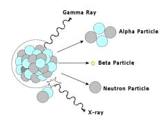
The four basic types of ionizing radiation are emitted from different parts of an atom, as shown in the image to the right.
