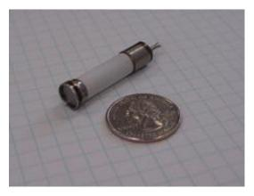
A current passed through a miniature coiled tungsten filament raises the temperature of the wire to approximately 1000°K, causing the thermionic emission of electrons. Typical currents of 5 to 100  $\mu$  amps of current are used depending on the type of analysis being conducted.
