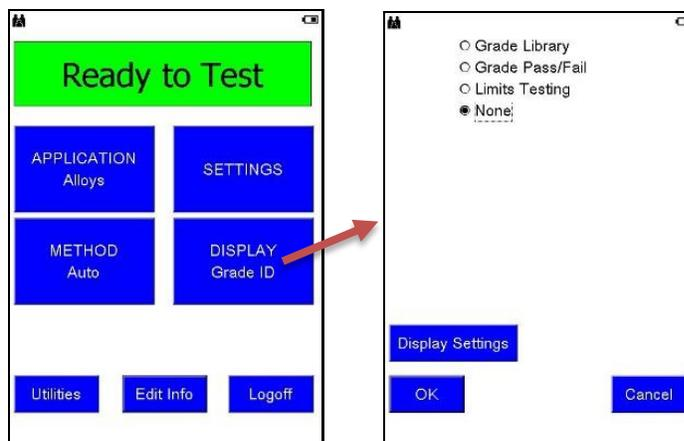
Limits Testing **Limits Testing** displays measurement results against minimum and maximum values. For more information, see *Restricted Materials Screening Application Guide*, Bruker document 030.0117 and *Soil Application Guide*, Bruker document 030.0118.
