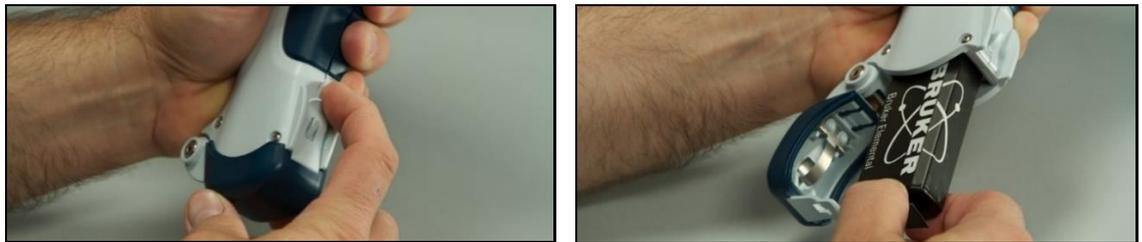
TRACER 5<sup>i</sup> battery removal
