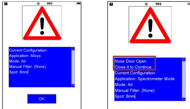
TRACER 5<sup>i</sup> open hatch If **OK** is not displayed, the hatch (little door in the nose) is open and the instrument is in an unsafe state. Close the hatch and the window closes.
