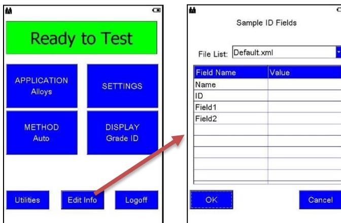
**Sample ID** Whatever is entered in the first field under **Value** is what is displayed in the **SampleID** field in Results (and the **Name** field in **Report Generator** in Bruker Instrument Tools). If **Operator** is the first value, then the second value is used for **SampleID**.
