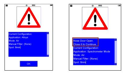
TRACER 5<sup>i</sup>If **OK** is not displayed, the hatch (little door in the nose) is open and the instrument is in an unsafeopen hatchstate. Close the hatch and the window closes.
