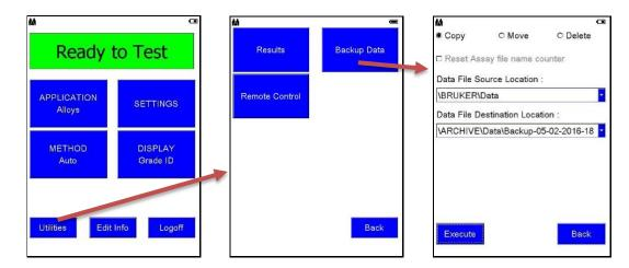
Reset counter When the **Reset the Assay file name counter** box is checked, if data are moved or deleted, the index counter resets to 1. This function is not available when **Copy** is selected.
