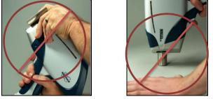
• Do not hold a sample by hand to the window for analysis. Hold the window to the sample.
