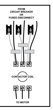
IF THE COIL VOLTAGE IS THE SAME AS THE LINE VOLTAGE AND THE CONNECTIONS TO THE COIL ARE EXTERNAL, WIRE THE COIL LIKE THIS:
