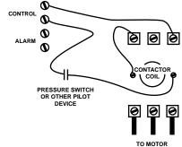
IF THE VOLTAGE TO THE COIL IS INTERNAL (FURNAS STARTER FOR EXAMPLE) WIRE THE COIL LIKE THIS:
