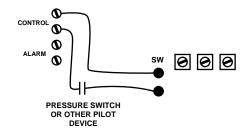
IF THE COIL VOLTAGE IS DIFFERENT FROM THE LINE VOLTAGE WIRE THE COIL LIKE THIS:
