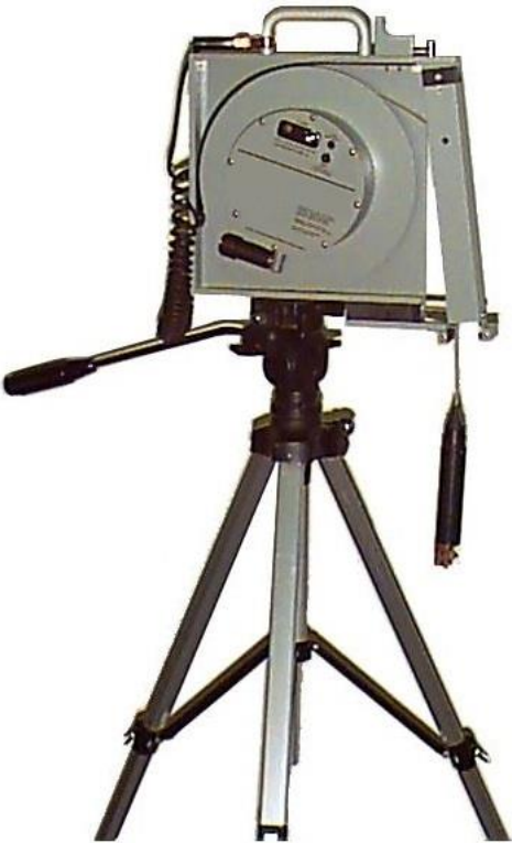
Example of Interface Probe Assembly mounted to tripod
